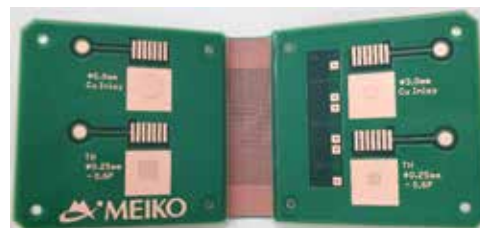
Multi-functional integrated power PCB (Downsizing, Large current, Heat dissipation, and 3D-Assembly)
