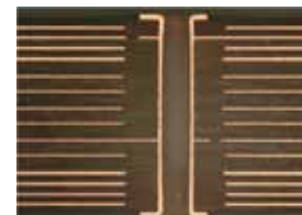
X-section of high speed material PCB
