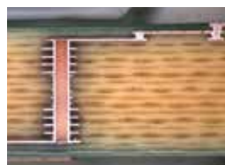
X-section of High Layer Count HDI PCB
