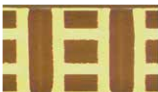
X-section of heavy copper through-hole PCB
