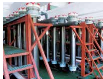
Photo: Soft etching waste liquid processing equipment in Guangzhou Plant.
