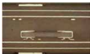
X-section of embedded passive devices PCB
